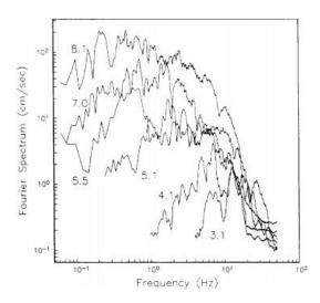
In Fig. example of Fourier Spectra of increasing magnitude accelerograms, recorded in 1985-1986 by digital instruments located on the Pacific coast of Mexico (Guerrero network).
